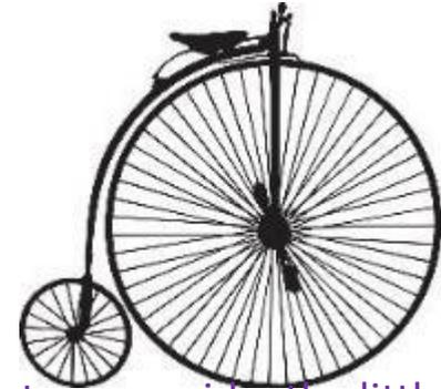
The perimeter or circumference of the small wheel is less. For every 100 metres you ride, the little wheel has to rotate more times than the large wheel
