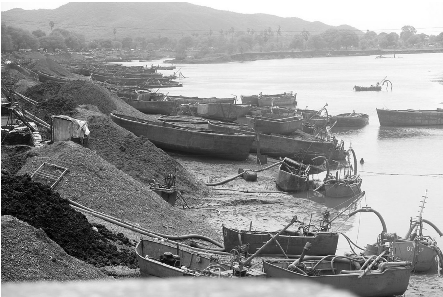
Figure 13.1 Suction pumps extract sand from a riverbank in India.
