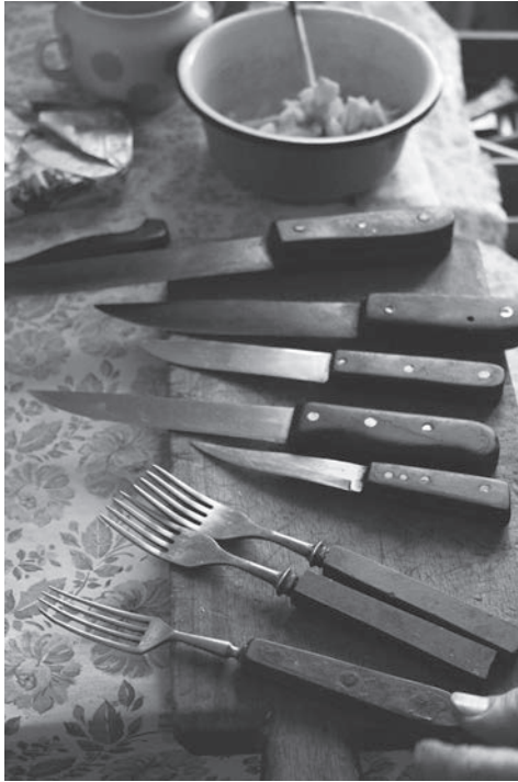
FIGURE 1.16. Knives and forks with simple black-ebonite handles, affixed at work. Top two knives are steel blades. Middle two: stainless steel self-made blades. Bottom: store-bought knife blade. Factory town near Leningrad, circa 1960s–1970s.
