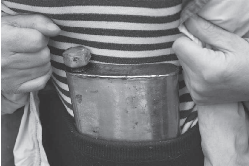
Figure 1.14. Flask. Made on a computer-operated lathe bench. Stainless steel. Leningrad, circa 1970s. Image courtesy Elena Tipikina.
