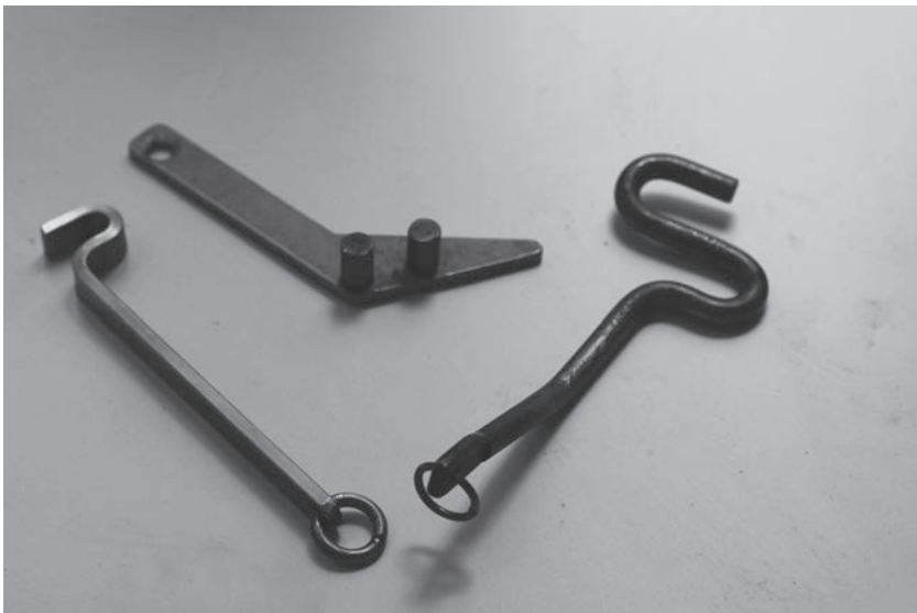
FIGURE 1.4. Three steel and titanium hooks, a rope-tow ski lift accessory. Gleaned from a classified institute in Leningrad in the 1960s.
