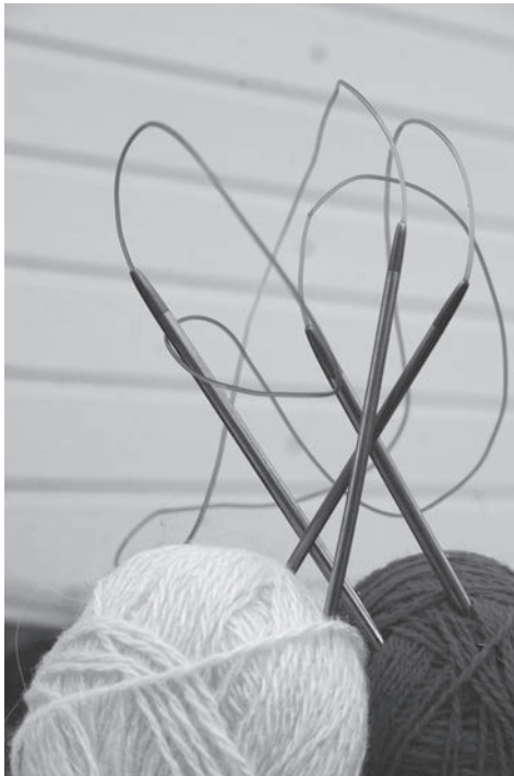
FIGURE 1.15. Four screw-top adjustable knitting needles. Made on a computer-operated lathe bench. Stainless steel, brass, fishing wire. Leningrad, circa 1970s. Image courtesy Elena Tipikina.
