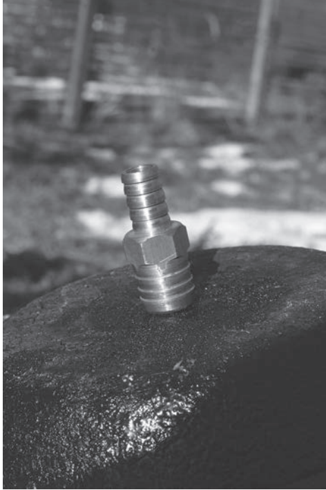
FIGURE 1.11. Brass nozzle, made by a lathe machinist at work. Image courtesy Elena Tipikina.
