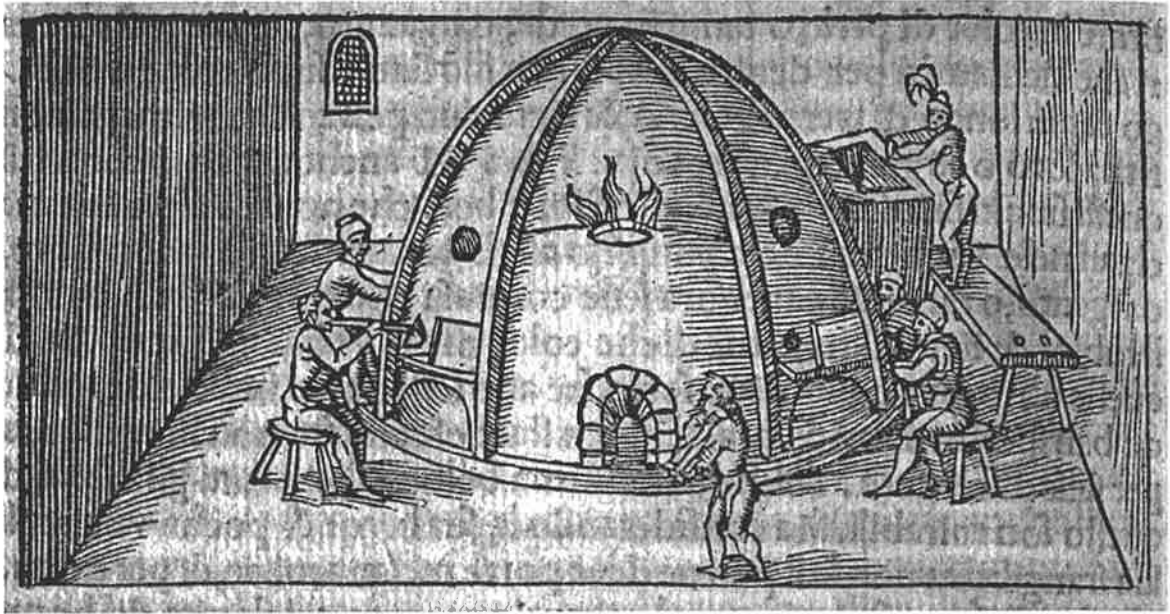
FIG 10. Glass furnace for melting and annealing, probably seen by Biringuccio during his visit to Murano. De la Pirotechnica (Venice, 1540) fol. 44.
