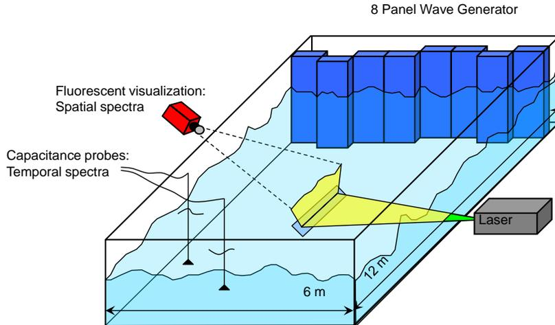
FIG. 2: Experimental setup, Total Environmental Simulator at “The Deep” Geography Department, University of Hull.
