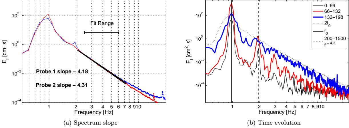
FIG. 7: Left: Estimate of spectrum slope for signal 352 in a trapezium flume with high driving rate. Right: Spectra before and after initial peak for signal 352 in trapezium flume with high driving rate. Behaviour is specific to case of high driving rate for experiments in a trapezium flume.
