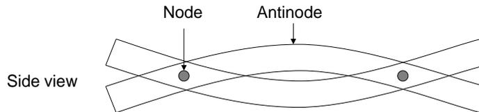
Energy is delivered by striking with a solid object (eg mallet). The length of time  $T$  that the head of a mallet is in contact with the body will influence the overtones produced, and frequencies  $f > 2/T$  will be damped. Soft mallets will deform more when struck and so will be in contact with the body for a longer time period : there will be fewer higher frequency overtones for a soft mallet than a hard mallet
