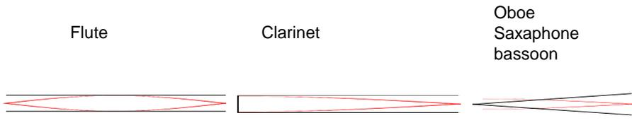
For a cone, wavefront is spread out over an increasing area
