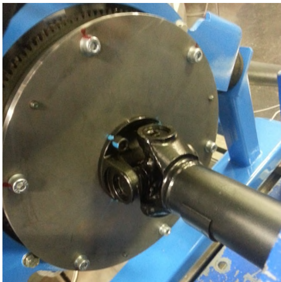
29 Jun 2016: Movement of mechanical fasteners at connection between propshaft flange and engine flywheel flange after limited running prior to rectification of issue.
