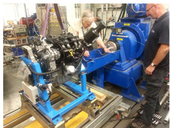
13 Jun 2016: WMG VEF technicians aligning the engine and mounting pallet with the dynamometer in the test-cell.
