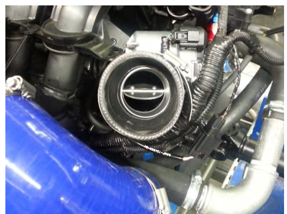
20 Jun 2016: Control of engine throttle established. Throttle plate near wide-open in this image.
