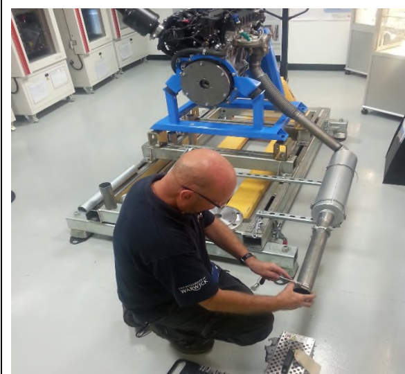
8 Jun 2016: WMG VEF technician trial fitting emissions gas analyser to the exhaust system.
