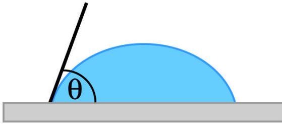
Again, for flat surfaces the measurement and baseline determination is fairly simple. However, for curved surfaces, a proper, curved baseline must be determined to provide an accurate contact angle.
