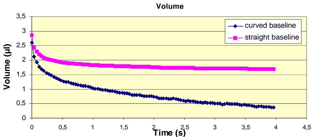
It can easily be seen that the uncorrected volume cannot be simply corrected or even approximated by subtracting off a constant volume in a linear fashion as might have been achievable with a reasonable approximation for the contact angle itself.
