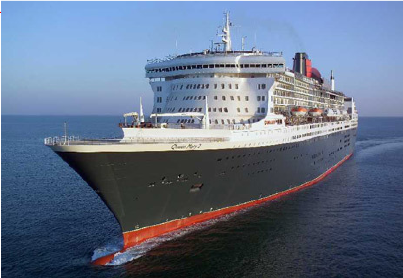
Queen Mary 2 - electric propulsion system: 4 pods totalling 86MW.
