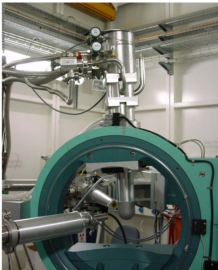
A view of the new low temperature ( >1.8K ) sample environment in operation on a recent user experiment. Also in the view, behind the Be dome of the cryostat, is the "tube slit" assembly. Both facilities have seen service in several user experiments.
