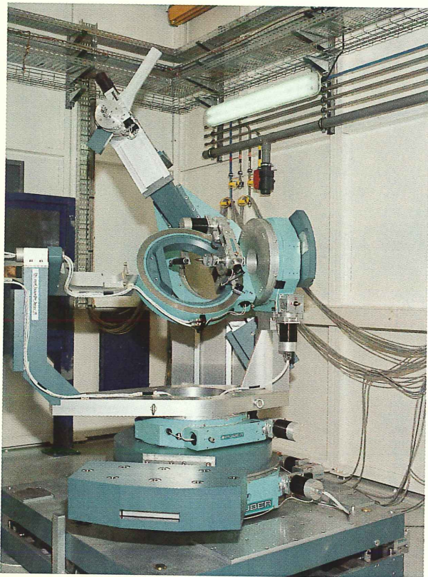
The XMaS 11-axis diffractometer which has recently been augmented by the addition of a polarisation analyser.
