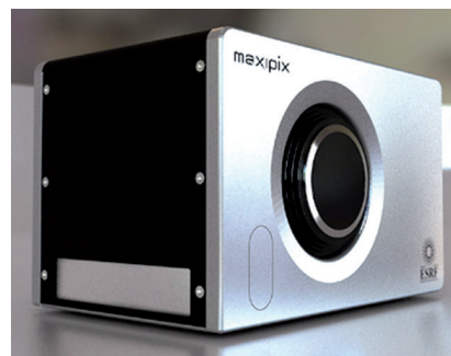
Fig. 7: Maxipix is a fast readout, photon-counting pixel detector system developed by ESRF and based on the Medipix2 readout chip developed by CERN and the Medipix2 collaboration. Image, courtesy of the ESRF-ISDD.
