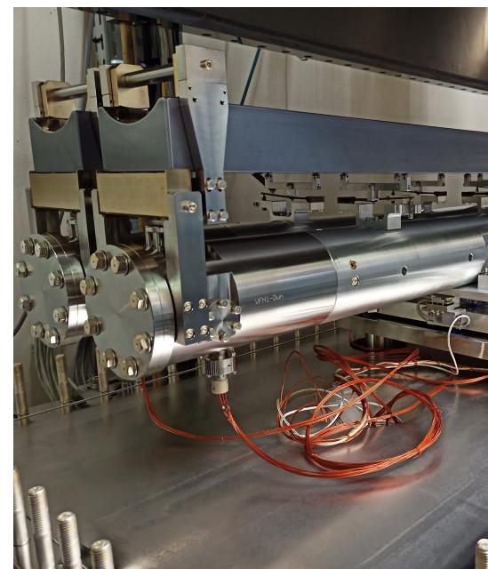
New double focusing mirror system with Cr and Pt coatings.
