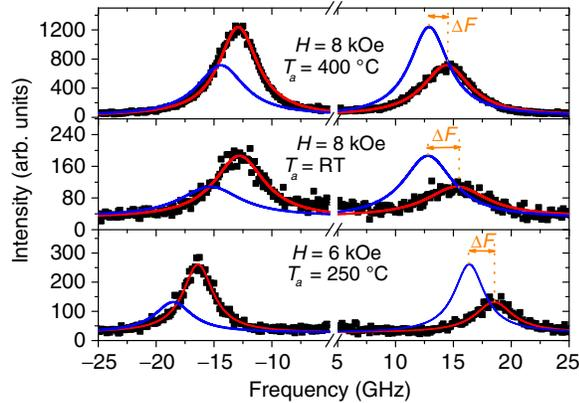
FIG. 7. BLS spectra of Pt/Co<sub>2</sub>FeAl(1.2 nm)/MgO grown on Si and annealed at various temperatures ( $T_a$ ) measured at 8 and 6 kOe in-plane applied field and for a characteristic light incidence angle corresponding to  $k_{\text{SW}} = 20.45 \mu\text{m}^{-1}$ . Symbols refer to the experimental data and solid lines are the Lorentzian fits. Fits corresponding to negative applied fields (blue lines) are presented for clarity and direct comparison of the Stokes and anti-Stokes frequencies.
