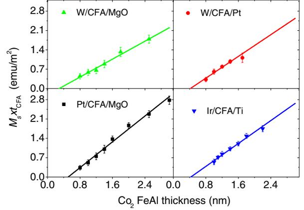
FIG. 1. Saturation magnetic moment per unit area versus  $\text{Co}_2\text{FeAl}$  thickness.  $\text{Co}_2\text{FeAl}$  thin films are grown on Si substrates with various buffer and capping materials. Symbols refer to the VSM measurements and solid lines are the linear fits.
