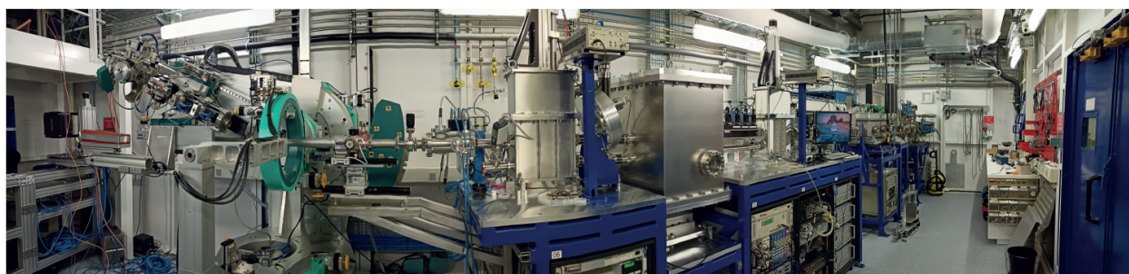
Figure A1: Panoramic photograph showing the experimental hutch of the XMaS facility. The beam enters from the right and proceeds via a series of in-line beam conditioning optics to the diffractometer (left).
