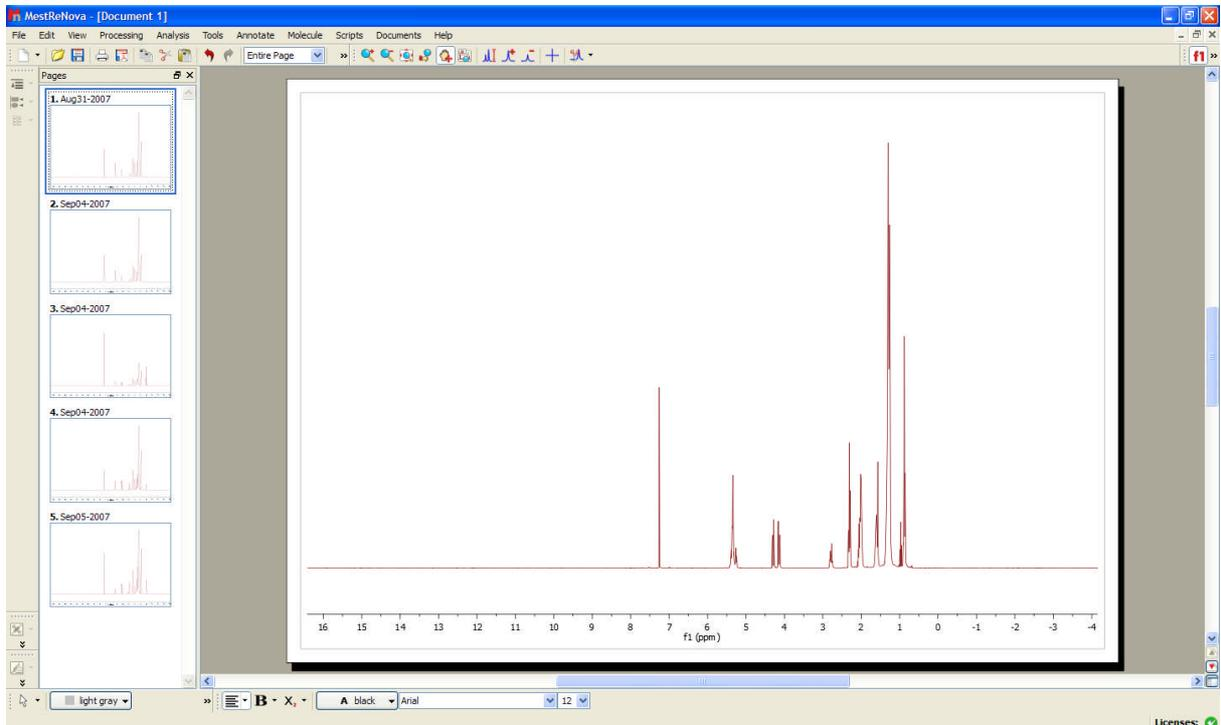
6. Select all of the spectra in the left hand column, and then click go to Tool > Stack Spectra. The spectra will be stacked in the order they appear in the column, with #1 being the bottom spectra and moving upwards.
