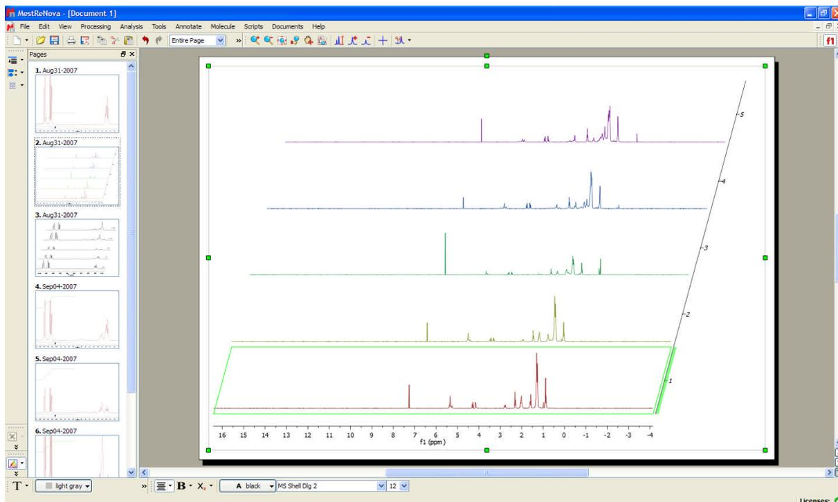
7. Select the stacked series of spectra and zoom in on the relevant area by setting the horizontal scale using the manual zoom button. Again, in this example, I have set the horizontal scale from 2.5 ppm to 4.5 ppm.
