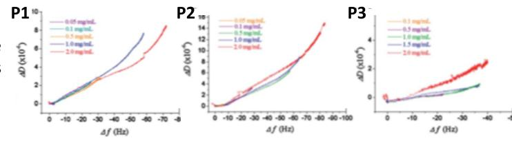
Large changes in dissipation ( $\Delta D$ ) indicate a flexible film, whilst small  $\Delta D$  values suggest a rigid, non-flexible coating: The longer chain polymer (P3) spans the binding site of ConA whereas the shorter polymers (P1/P2) can only bind one site.
