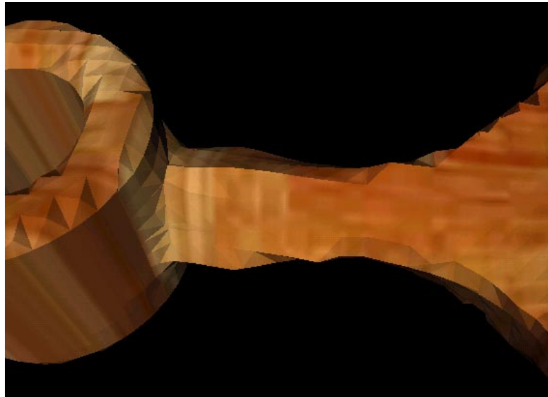
Figure 8.15: Image of the curtain pole support with a twisted neck.
