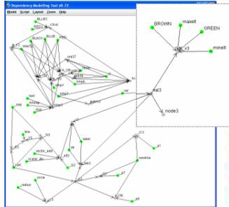
The nodes in the inset at the top right express the dependency that accounts for the colours of the array elements: the largest is displayed in brown, the smallest in green, the others in blue.
