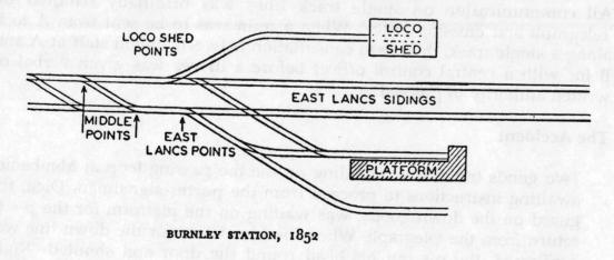
The station is a terminus for a single line. It has no signals, and all the points are manually operated. The East Lancs Points are normally set to the platform, and are weighted in such a way that they have to be held in position with a lever in order to direct trains into the East Lancs
