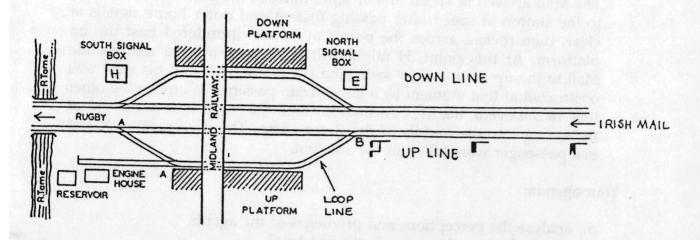
The station caters for express trains that don't stop, but the points can also be set so that trains can stop at the platforms. The points at A are interlocked so that when they are set for an express train they are also automatically set for the siding that leads to a dead end near the engine house.
