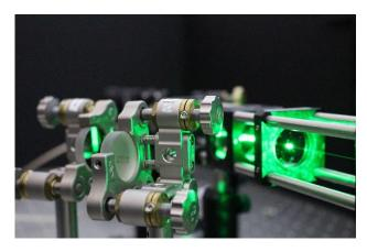
We send in green light to excite a single NVC, polarizing its electron spin, before using magnetic resonance to control its quantum state and then detecting its final state by measuring the red florescence it emits.
