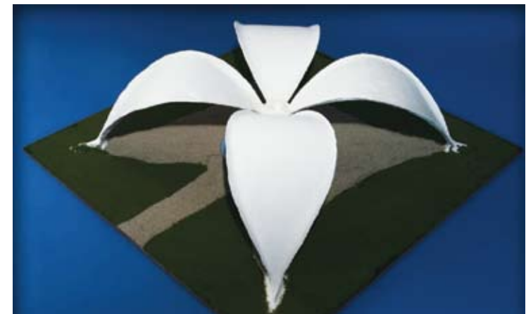
» Inverted rigid shape giving a shell structure
