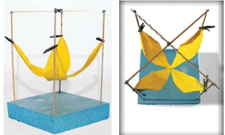
» Fabric hanging model prior to being 'frozen' in a rigid material
