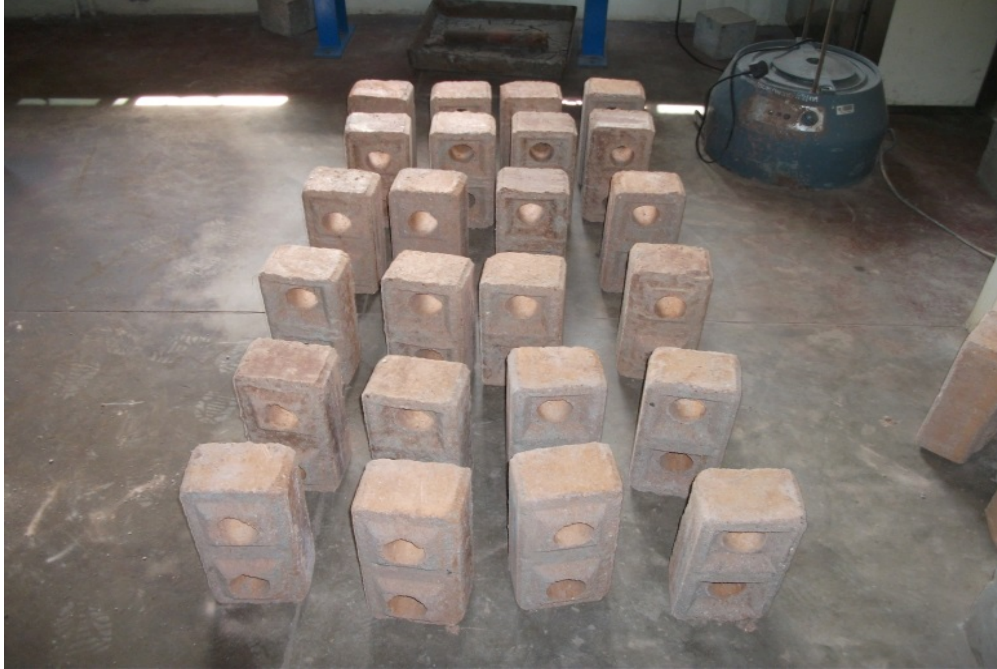
Figure 2: ISSB Used for Compression Testing
