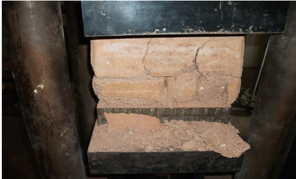
Figure 4: Crushing failure of sample
