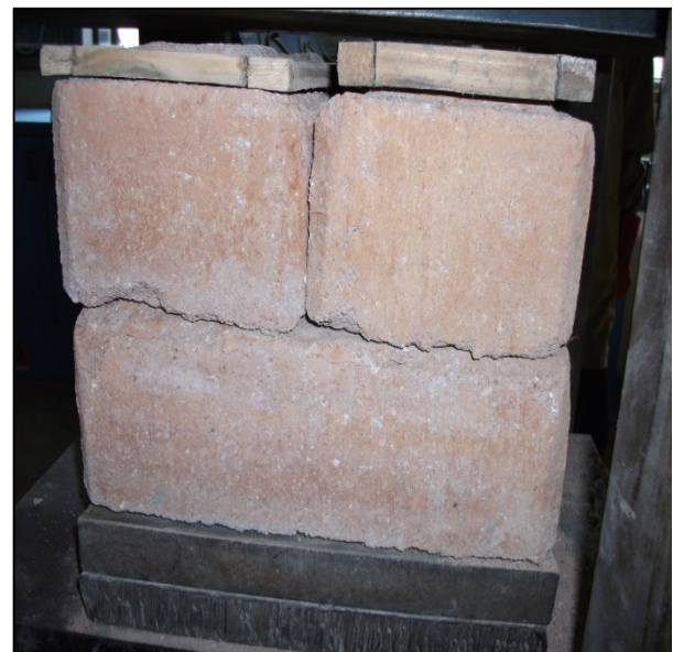
Figure 3: Setting of sample in testing machine
