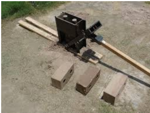
The Cinva ram machine for production of compressed mud bricks
