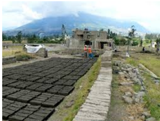
The best compressed mud bricks comes from clayey soils
