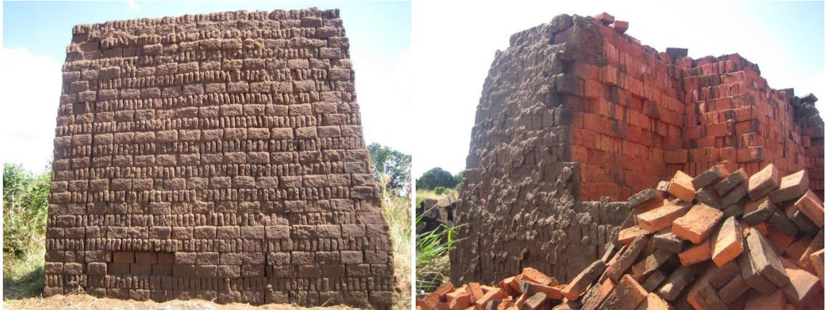
Figure 4: Bricks within 300mm of the clamp kiln's surfaces have a very low quality (Tanzania).
