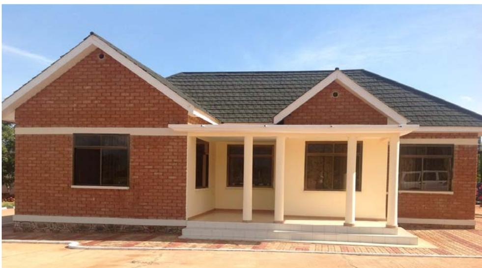
**Fig. 1** Tanzanian House made of Mortarless Interlocking Blocks of Stabilised Soil.
