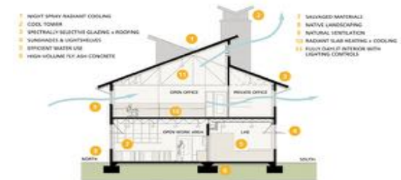
Enhanced stack effect ventilation, Global Ecology Center, Washington
