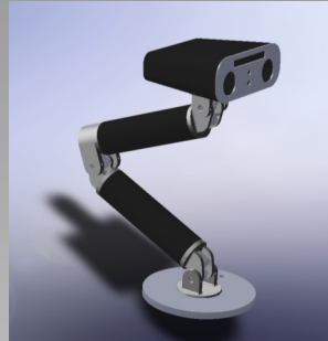
Right: Concept carbon fibre arm design
