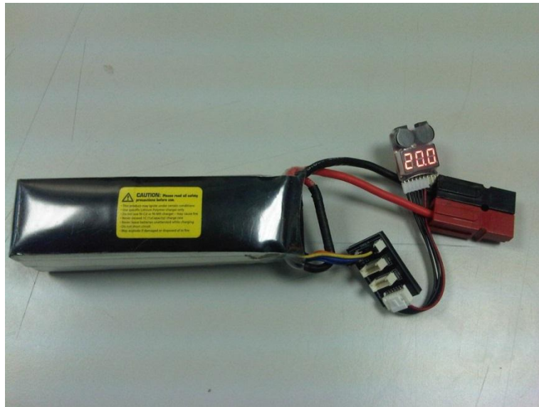
Figure 60: Battery with attached LiPo warning circuit
