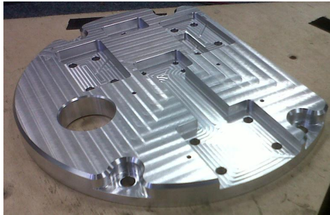
Figure 33: Base Plate - Two Set-ups and Three Tool Changes
