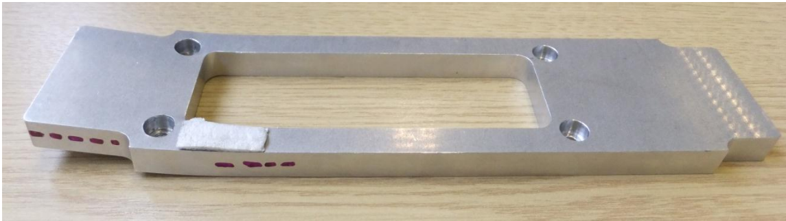
Figure 77: Distortion in flipper motor housing
