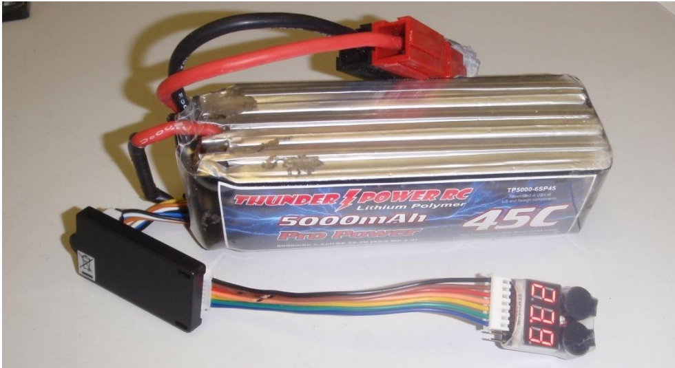
Figure 38: Photo of the original battery monitor
