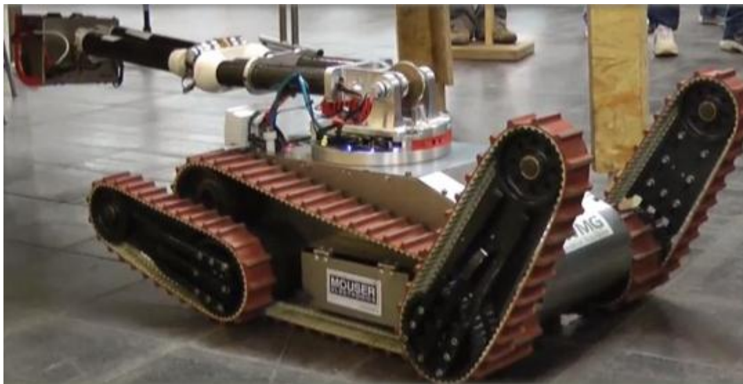
Figure 66. Robot in "limbo" position under a low table.
