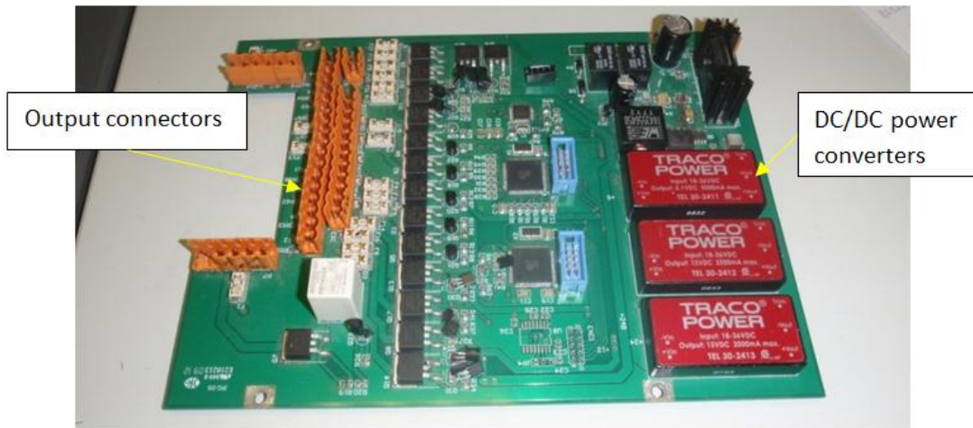
Figure 40: Photo of the original power board
