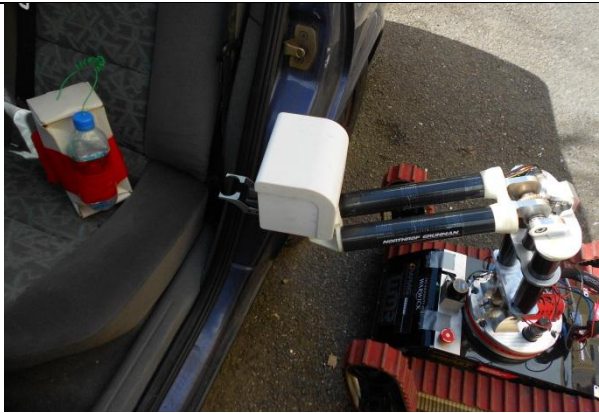
Figure 77. Blind gripper test from car seat
