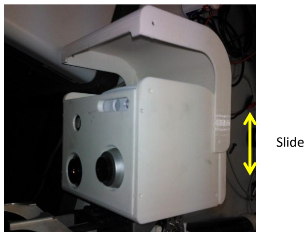
Figure 51. Sliding lid for easy access to internal components.
