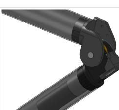
The robot's arm has been redesigned to provide additional degrees of freedom at the end effector, allowing better positioning of the new manipulator. The redesign is also serving as an opportunity to better design the arm joints to shield gearing and positional feedback components and to reduce some of the looseness and subsequent positional ambiguity found in the current arm.
