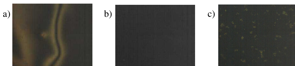
Figure 4.1. Microphotographs of samples viewed under crossed polarisers, magnification \times 250 . Alignment direction along one of the polarisers. Host material 5CB.
