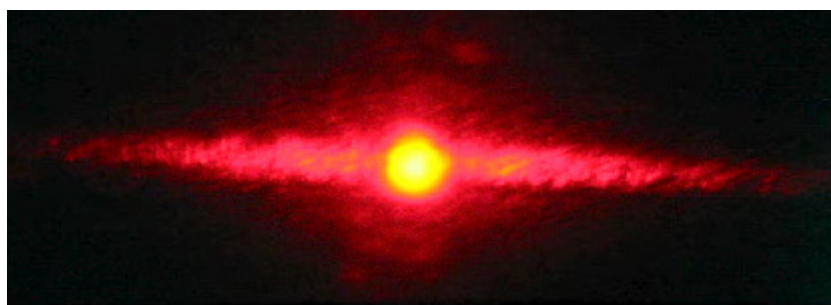
Figure 6.5. Scattering of the reading beam on a sample (device 31, C_{60} doped BLO48) with applied 5V_{DC} . The device is planarly aligned, and the alignment direction is vertical. To avoid interference from the scattering, a horizontal grating should be recorded, so that the diffracted orders are above and below the main order, not on the sides.
