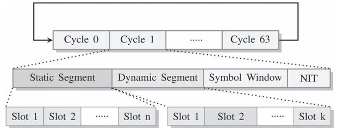
Fig. 1. FlexRay communication cycle.
