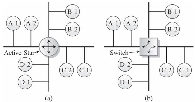
Fig. 2. (a) Standard and (b) switched FlexRay network topologies.
