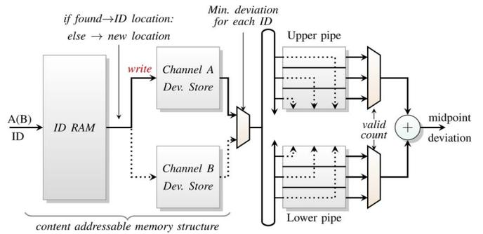
Fig. 9. CAM organization and fault-tolerant midpoint computation for offset correction.
