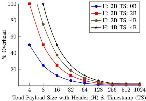
Fig. 17. Overheads for including headers and timestamps.
