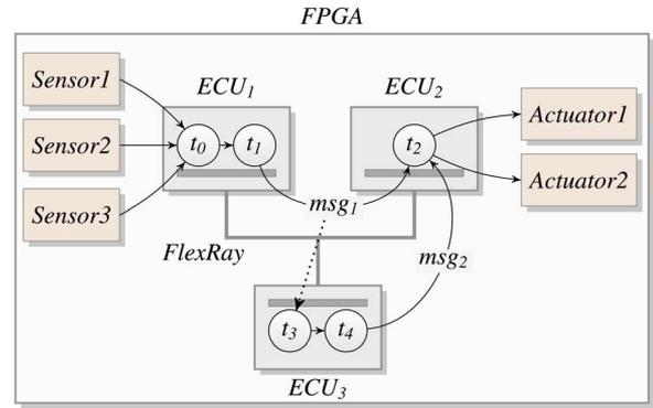
Fig. 13. Test setup for brake-by-wire system.
