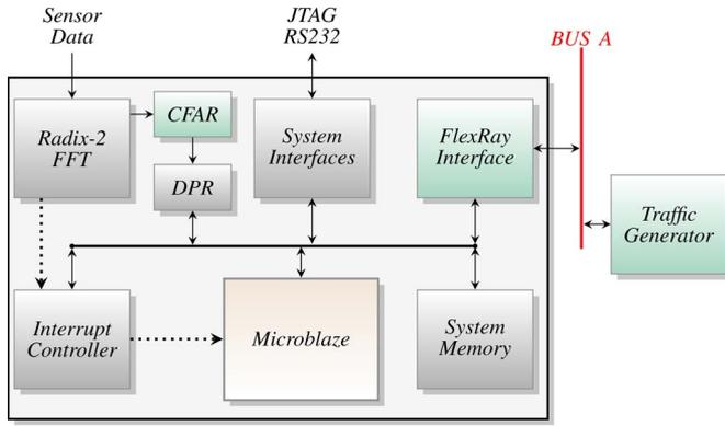
Fig. 12. Integrated ECU function on Spartan-6 FPGA.
