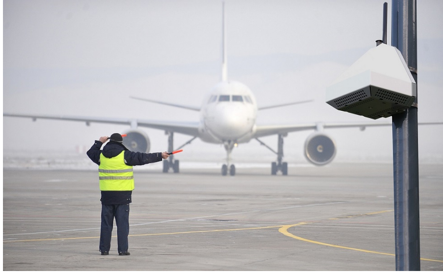
Figure 2.2: An example of a low-cost air quality monitoring device called AQmesh installed at an airport (donated by Environmental Instruments Ltd.) [82].
