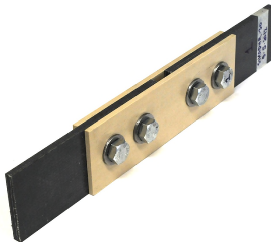
Resin injected test specimen ready to be tested
