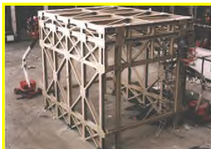
Large frame is electrically non-conductive, 1996
