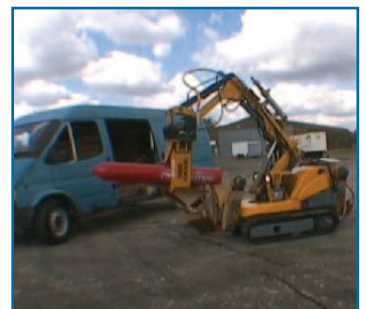
Photo 1 – An ROV gains access before searching and identifying types, sizes and ownership of the cylinders inside.
