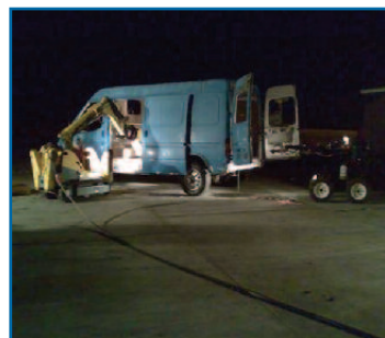
Photo 1 – An ROV gains access before searching and identifying types, sizes and ownership of the cylinders inside.
