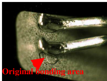
Figure 17: An example for bond wire lift off [Johnson05]
