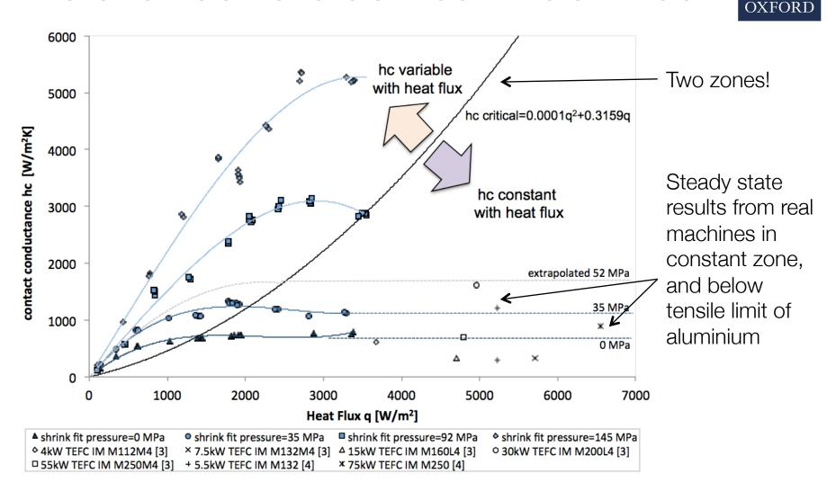
Camilleri R, Howey DA, McCulloch MD, "Experimental investigation of the thermal contact resistance in shrink fit assemblies with relevance to electrical machines", IET PEMD, 18-20 April 2014, Manchester UK.
