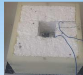
Test rig measures sample's thermal conductivity
