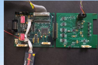
FPGA control boards
