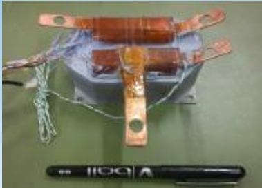
Potted inductor with embedded thermal sensors
