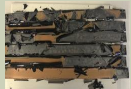
Catastrophic insulation degradation of samples at 260°C after 1600 hours
