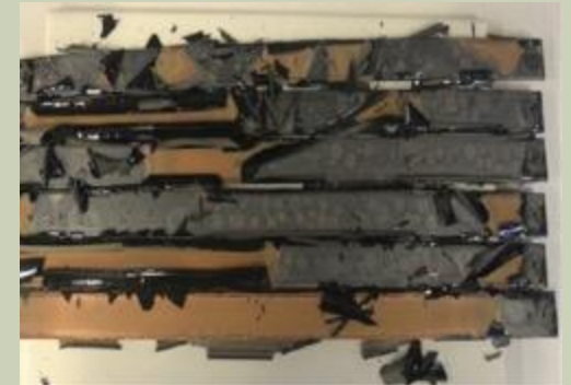
Catastrophic insulation failure of samples at 260°C after 1600 hours
