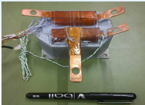
Potted inductor with embedded thermal sensors
