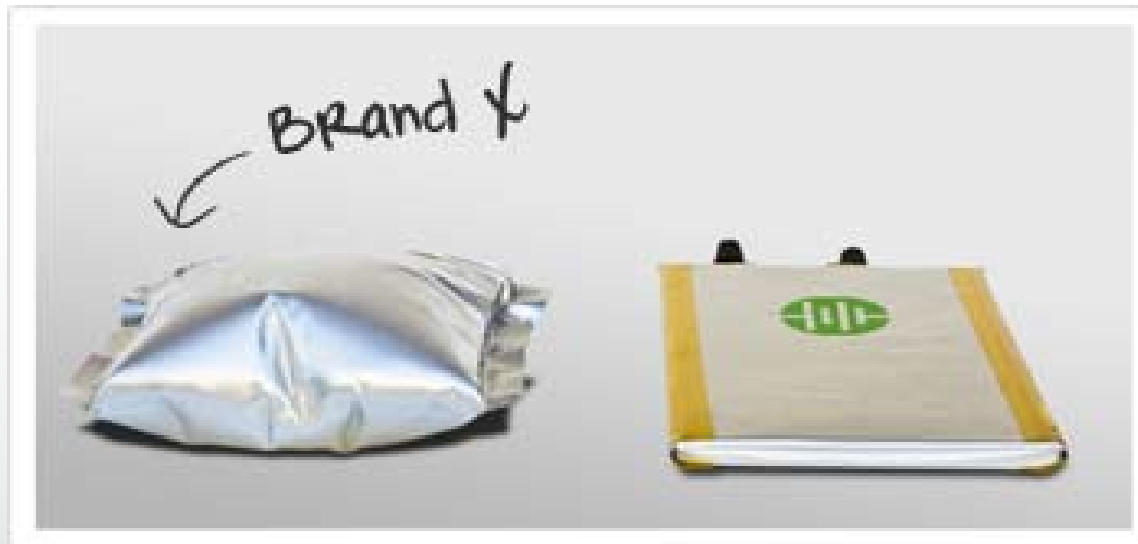
Figure 1: Gassed and normal Li-ion pouch cell
