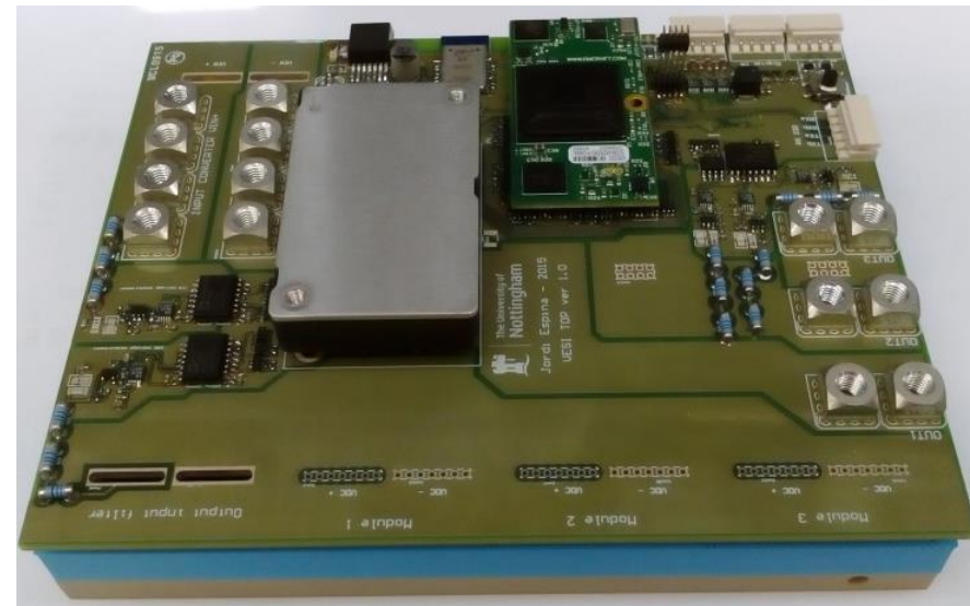
DC-DC power converter, 300V In, 0-250V out, 52kW max rated power (12.8 x 16.3 x 3.3 cm)
