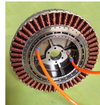
Stator for in-wheel rare-earth PM motor
