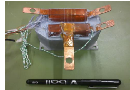
Interleaved DC-DC converter inductor incorporating gap loss mitigation
