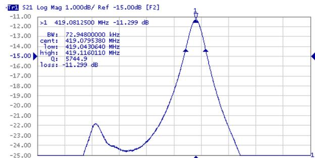
Fig. 10. Frequency response of an extended cavity Au RSAW sensor device with improved TWGM suppression. Horizontal scale: 100 kHz/div.
