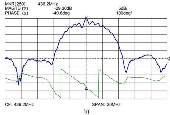
Fig. 3. Frequency (upper plots) and phase (lower plots) responses of a two-port RSAW resonator with Au metallisation and strong excitation of a parasitic SSBW mode. The broadband responses (a) indicate the lower-frequency RSAW mode at about 436 MHz and the SSBW mode at about 70% higher frequency. The narrowband RSAW responses (b) indicate very weak resonance behavior (ripples) on top of the  $\sin(x)/x$  response of the IDTs.
