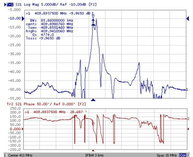
Fig. 11. Frequency (upper plot) and phase (lower plot) responses of an Au RSAW inline coupled dual mode resonator filter with increased phase slope within its pass band.
