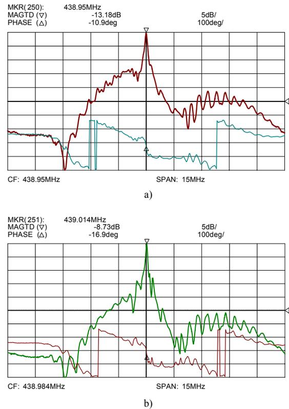
Fig. 8. Comparison of two identical Au devices (a) with and (b) without random interruption of the reflector fingers according to Fig. 7. Upper and lower data traces are the device frequency and phase responses, respectively.
