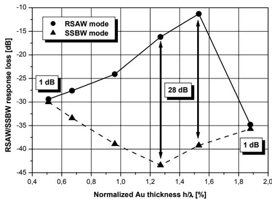
Fig. 5. Insertion loss behavior of the RSAW and SSBW modes versus Au thickness for the device from Fig. 3 and 4.
