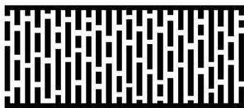
Fig. 7. Reflector with randomly broken fingers for TWGM suppression.
