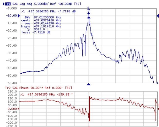
Fig. 6. Frequency (upper plot) and phase (lower plot) responses of a low-loss thickness optimized Au RSAW two-port resonator with  $85\lambda$  aperture for strong load coupling. Horizontal scale: 1.5MHz/div.
