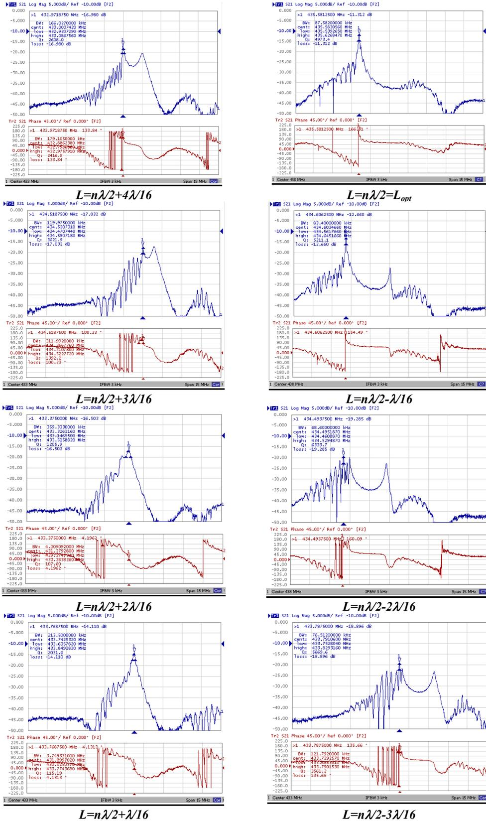
Fig. 9. Spacer variation in the device from Fig. 6. The upper and lower data plots are the frequency and phase responses, respectively.
