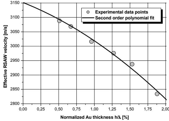
Fig. 2. Effective RSAW propagation velocity in a two-port resonator with Au electrode structure versus normalized Au film thickness.
