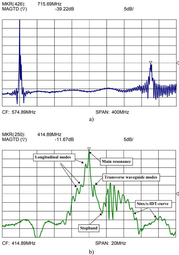
Fig. 4. Broadband (a) and narrowband (b) frequency response of the device from Fig. 3 with an Au thickness optimized for maximum coupling at the RSAW mode and highest suppression at the undesired SSBW mode.
