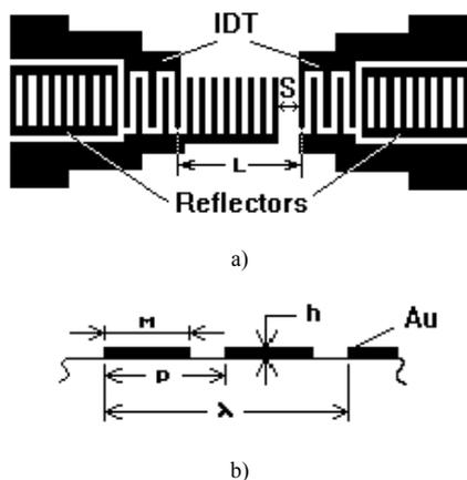
Fig. 1. Geometry (a) and metallisation parameters (b) of a RSAW based two-port resonator with Au electrode structure.
