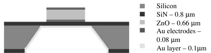
Fig. 1: Cross section of the FBAR sensor.
