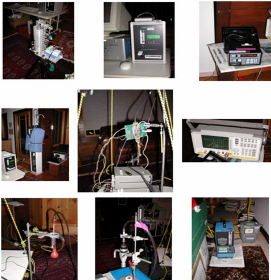
Figure 4.25: Field test instrumentation. Top row (L to R): Quartz crystal microbalance (QCM); Aethalometer; optical particle counter (OPC). Middle row: High-flow sampler for measuring episodic source-enriched PM 2.5 ; MEMS PM monitor; spectrum analyzer displaying FBAR resonance. Bottom row: Bubble flowmeter for use with MEMS PM monitor; FRM sampler for PM 2.5 ; pump and gas meter for FRM sampler.
