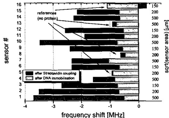
**Figure 5. Measured frequency shifts at 25°C caused by the attachment of bio-molecules to FBAR sensors of different area, using biotin-labeled DNA oligos as a receptor and streptavidin as the target protein.**
