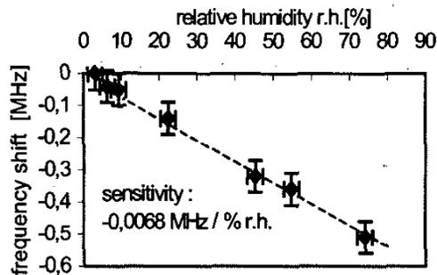
Figure 6. Frequency shift of an FBAR with 200  $\mu\text{m}$  diameter coated with a 50 nm thick humidity absorbing polyimide.
