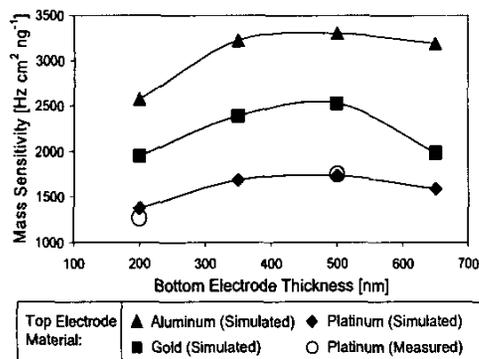
**Figure 4. Variation of mass sensitivity with bottom electrode thickness and material of the 100 nm thick top electrode. Simulated and measured values for devices with Pt top electrodes show good correlation.**
