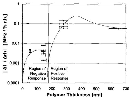
Figure 7. Measured sensitivity to relative humidity versus the thickness of a humidity polymer covering 1.6 GHz FBAR sensors, compared to simulation data (line).
