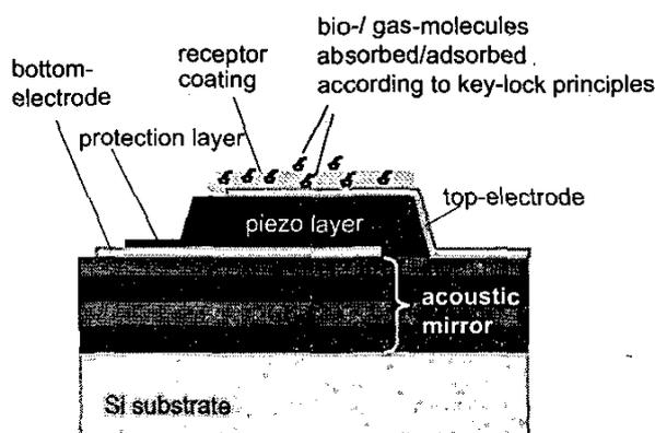
Figure 1. Schematic of the FBAR bio- and gas-sensor. The principle relies on a resonance shift caused by the attachment or absorption of molecules to a receptor coating covering the surface of a thin-film resonator.
