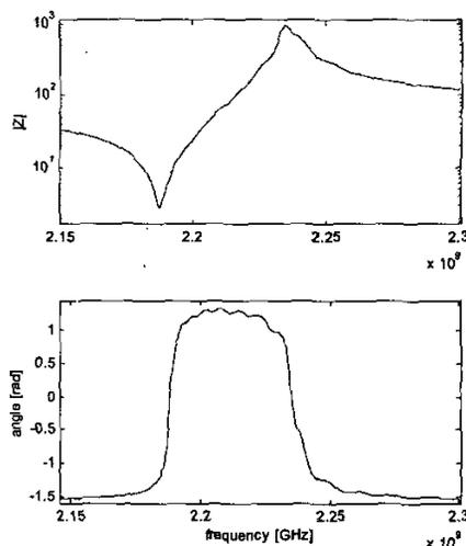
Figure 3. Measured impedance characteristics for a resonator of  $70 \times 70 \mu\text{m}^2$  area exhibiting a Q-factor of more than 400 in both series and parallel resonance.
