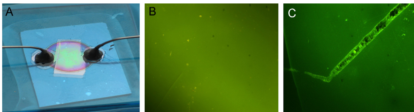
Fig. 5. Images of the basic element of a lab-on-chip based on a PSi optical transducer: (A) a real view of the porous hybrid silicon-glass chip; (B) fluorescent images of labelled proteins; (C) particular of a scratch on the chip surface.
