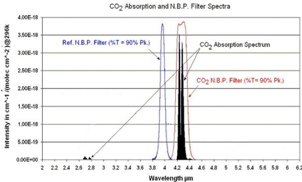
Fig. 1. CO<sub>2</sub> absorption spectrum and filter cutoff wavelengths.
