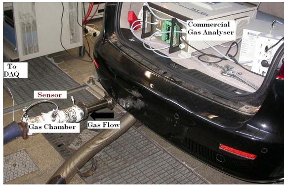
Fig. 4. Photo of the engine test setup carried out in facilities in Centro Ricerche Fiat, Italy.
