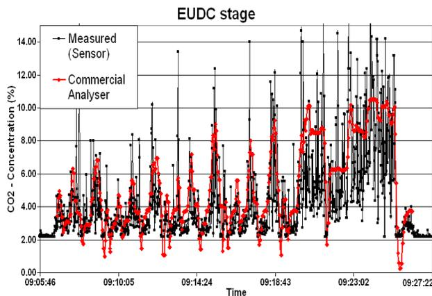
Fig. 5. Measured concentrations from the sensor for the EUDC test cycle on a Fiat Croma engine exhaust. Also shown are the equivalent recorded concentrations from the commercial analyser.
