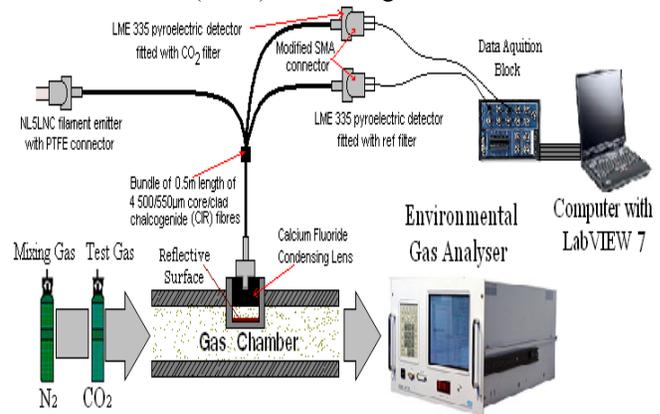
Fig. 2. Mid-infrared optical fibre CO<sub>2</sub> sensor.
