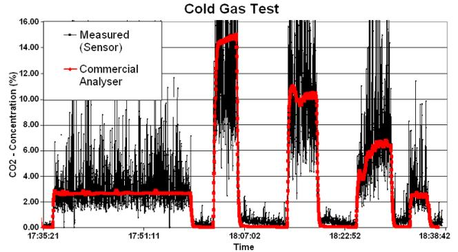
Fig. 3. Shown is the response from the sensing system to the initial cold gas test, also shown are the equivalent recordings from the commercial gas analyser.
